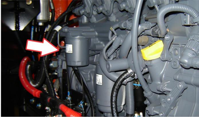
Lube Point(s) - Fill Cap/Spin-on Element
